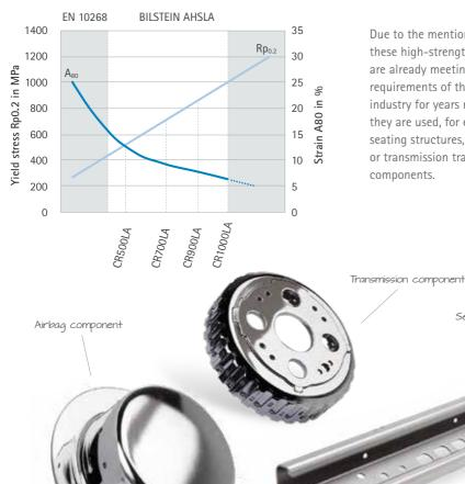
Due to the mentioned properties these high-strength materials are already meeting the high requirements of the automotive industry for years now. Currently they are used, for example, in seating structures, airbag systems or transmission transmission components.
