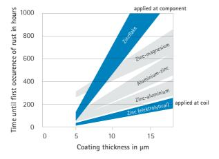
To protect the surfaces, metallic coatings can be applied electrolytically to the coils. Alternatively, highly corrosion-resistant zinc flake coatings as well as wet and powder coatings can be applied to the component or final product.
